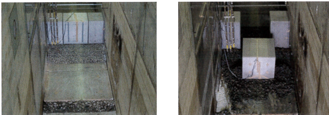
Figure 10 Large-scale hydro flume experiment of Arikawa and Shimosako (2013), showing views before and after the experiment. Caisson failed accompanying flow deformations of the rubble mound under tsunami
