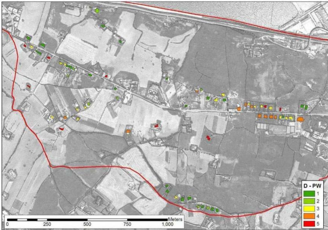
Figure 3.12. Observed damage to perimetral walls
