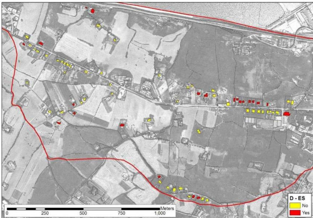
Figure 3.15. Observed damage to external staircases
