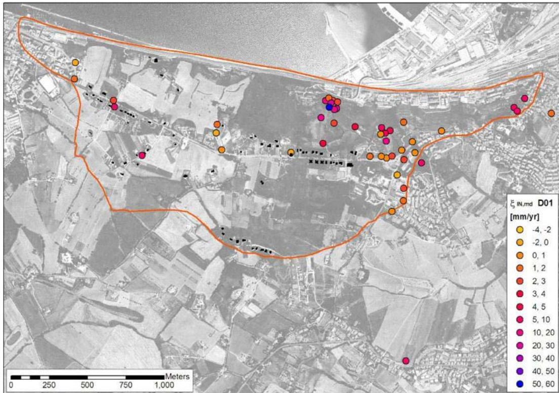
Figure 3.32. Inclinometer-based estimates of \xi_{IN,md} at reference depth D01.
