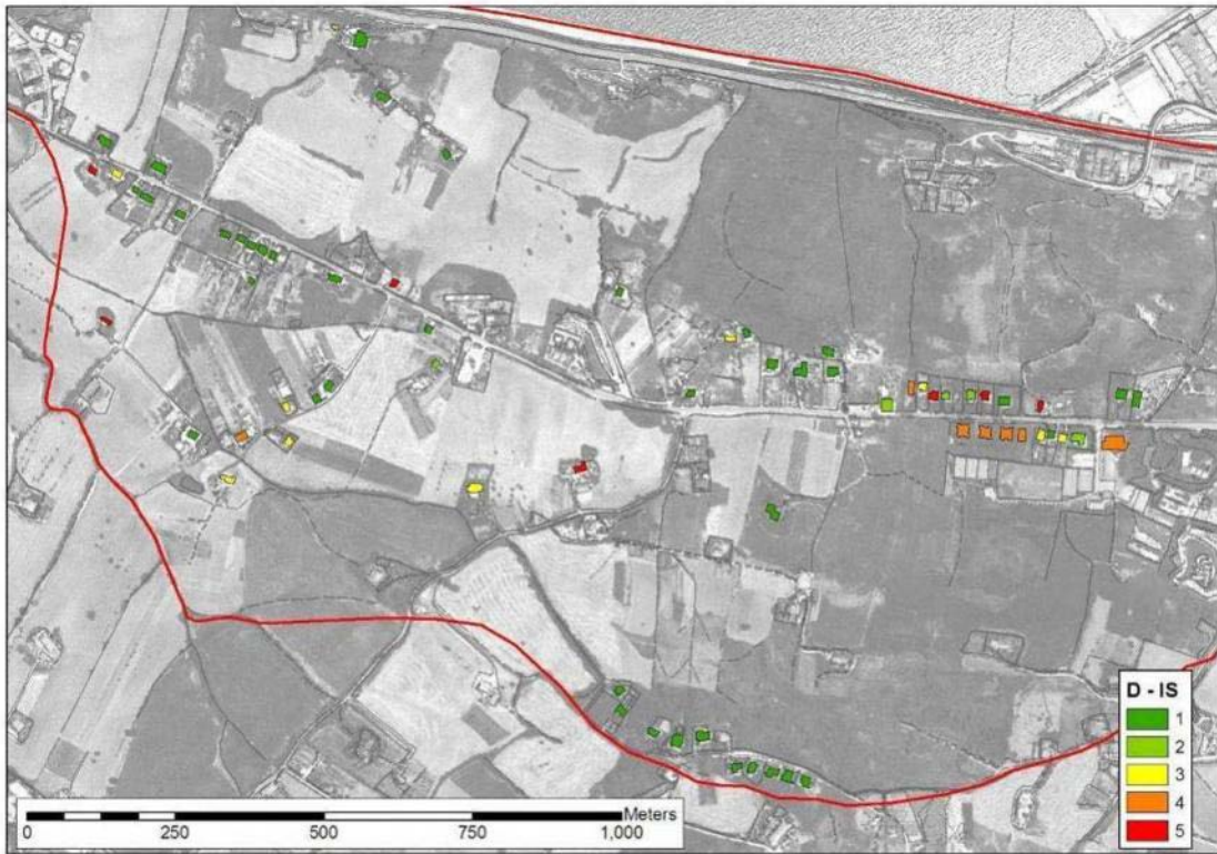
Figure 3.14. Observed damage to internal staircases
