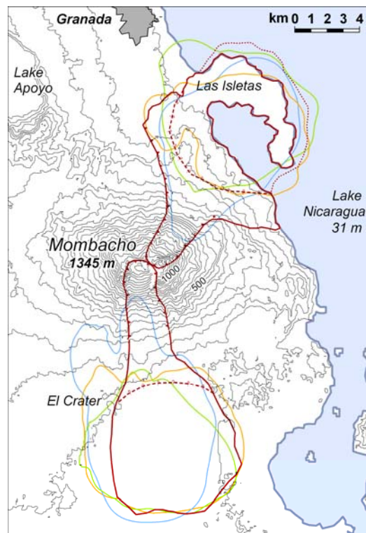
Figure 4.6.4 - Outline map of the debris avalanche deposits obtained assuming the frictional (green), Voellmy (orange), and plastic (blue) rheologies compared against the debris-avalanche deposits from the field data (in brown).
